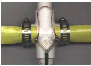
frequency) when the two elements were spaced approximately 1 inch apart. Figure 1 shows the method used to attach the driven element to the PVC cross.
