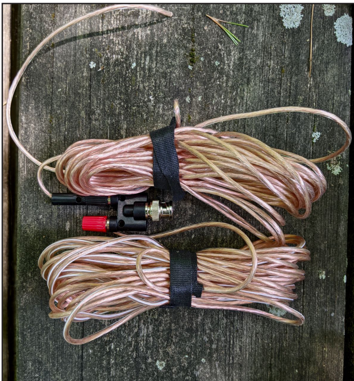
Figure 4: My new speaker wire antenna in all its glory.
