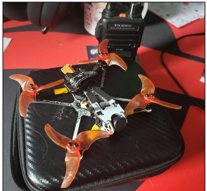
This is the Emax Tinyhawk 2 Freestyle, a pre-built bind and fly quadcopter. It’s small (note the Yaesu FT-65 for scale) but it will bind to a quality RC controller and have you flying (and crashing) in no time!
