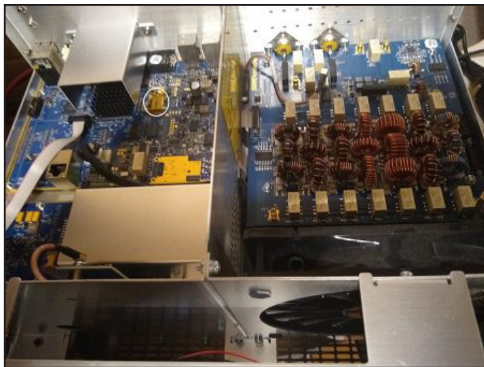
Inside the Flex 6400. At the lower right is the fan. Circled is the SD card referred to in the text.
