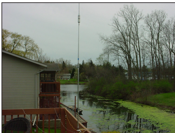
A view of the 40-meter “Ham Stick” and small radial package
