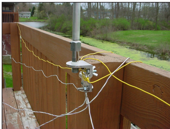
A close-up of the feedpoint and the radial wires.
