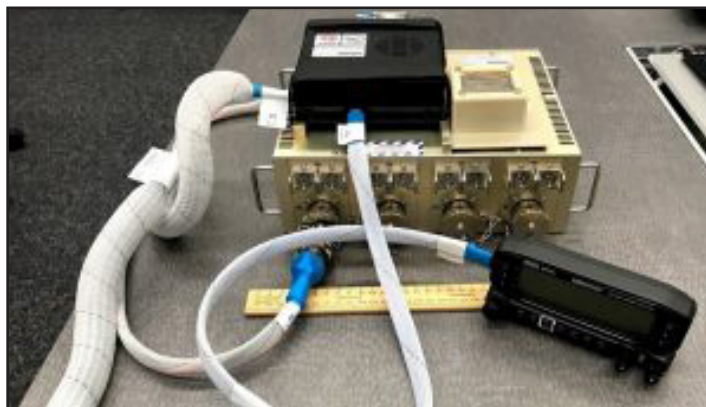
This recently-installed ham gear on the ISS includes a V/U crossband repeater.
