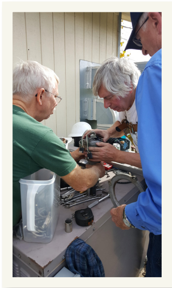
After discovering the rotor would not turn, Steve (W8RQS), Tom (WA8WPI), and John (KE8CYC) opened the bottom to discover the chain had slipped off the gear.
