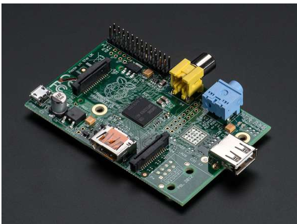
Raspberry Pi Model A: A single board computer the size of a credit card. It weighs approx. 1oz. and measures 2.5" x 3.63" and is 0.58" thick
