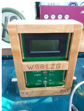
Great Find: Homebrew SWR Meter with custom wood case by Gregg Mulder/ WB8LZG
