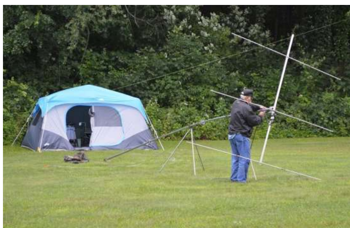
Jim/KA8DDQ assembling his 6m Yagi for the VHF Station
