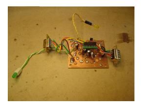
$2^{nd}$  step, mount the 5 caps, 1 diode, 3 resistors, 2 LED's, and connectors.  $3^{rd}$  step, finding an encloser. I had some extra Ten Tec style boxes in my "junk box", so I started drilling the holes for the jacks and LED's.
