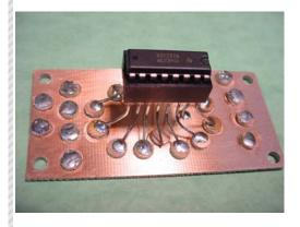
It is built ala "Manhattan style" with only a handful of parts around a MAX232 chip, it is a great way to get your rig up and running on computer control.
