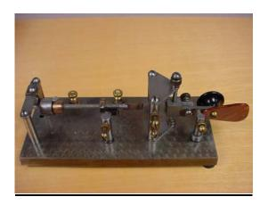
The Key of the Month for April is a one of a kind homebrew bug. This key was a replica of the famous Vibrboplex "Lightning Bug". The craftsmanship is superb, and the bug handles very well. In fact, it will send better at slower speeds than a Lightning Bug, because it has a slightly longer pendulum. The key was purchased in Grand Rapids from a SK in the early 1990's, and is a testament to the FB work and attention to detail of machinists in an era gone by.
