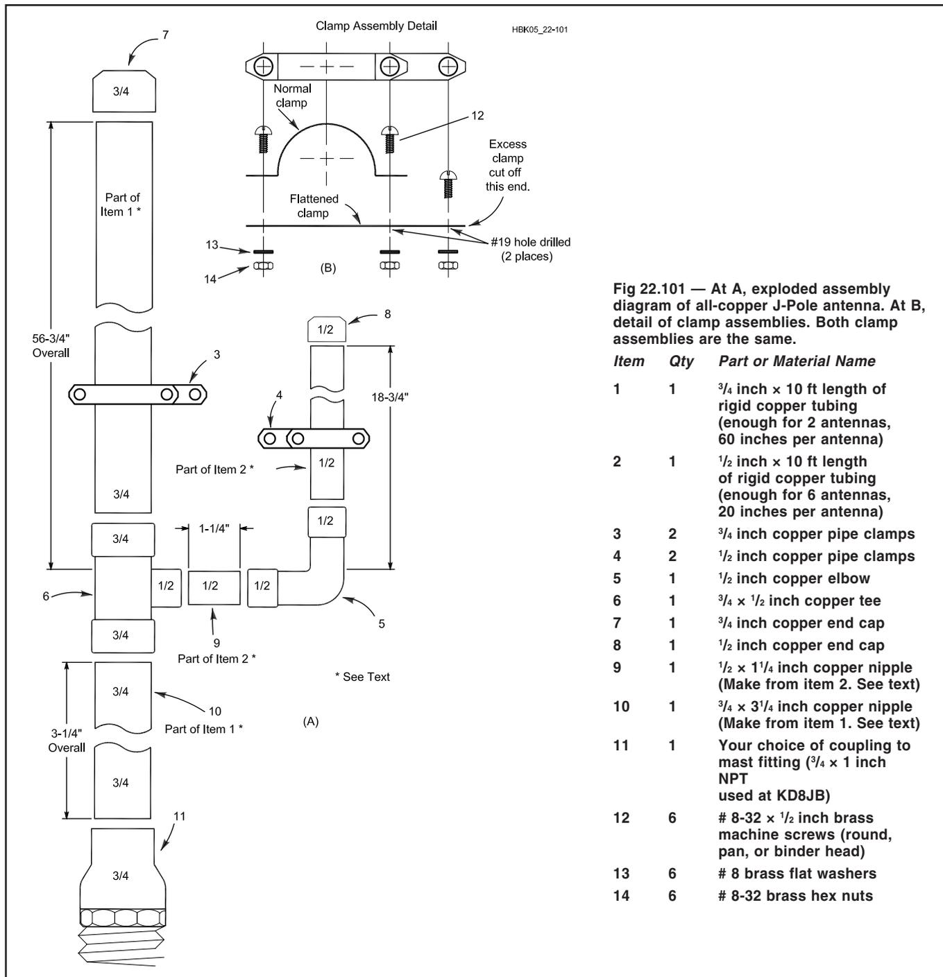
**Fig 22.101** — At A, exploded assembly diagram of all-copper J-Pole antenna. At B, detail of clamp assemblies. Both clamp assemblies are the same.
