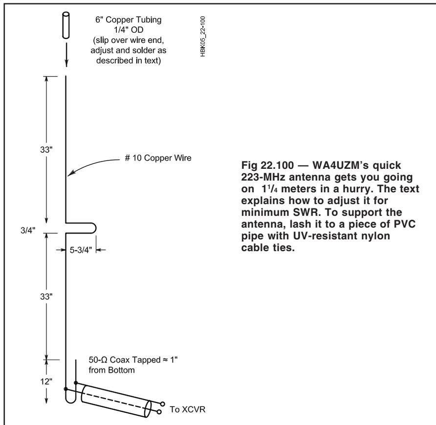
**Fig 22.100** — WA4UZM's quick 223-MHz antenna gets you going on 1 $\frac{1}{4}$  meters in a hurry. The text explains how to adjust it for minimum SWR. To support the antenna, lash it to a piece of PVC pipe with UV-resistant nylon cable ties.
