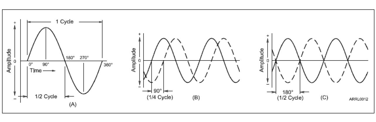
Position within a cycle is called *phase*. Phase is used to compare how sine wave signals are aligned in time. Measured in degrees.
