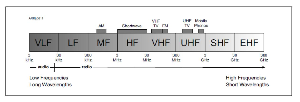
Signals that have a frequency greater than 20,000 Hz (or 20 kHz) are *radio frequency* or RF signals.
