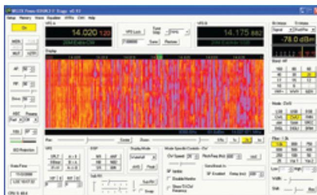
Figure 2 — Lower 40 kHz of 20 meters as a waterfall display.
