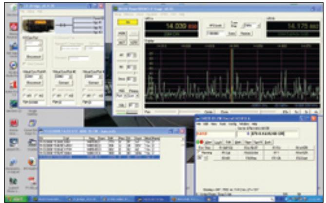
**Figure 4 — Demonstration of *LP-Bridge* providing simultaneous serial access to both *PowerSDR* and the N1MM contest logging program. Two other applications can also share the data from the K3 serial port without interfering with each other.**
