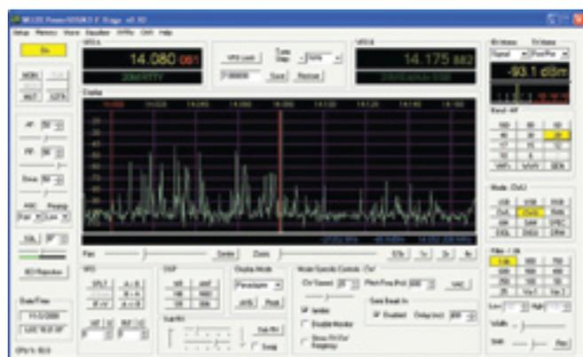
Figure 1 — Wideband panoramic view of the CW portion of 20 meters during the 2008 ARRL CW Sweepstakes.
