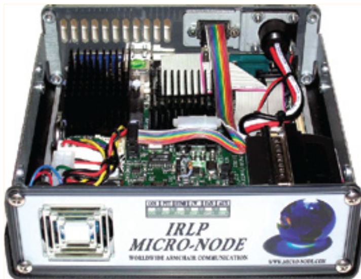
Figure 6 — The Micro-Node MN-1000 stand-alone embedded system measures only 2.4 × 6.9 × 7 inches and is ready to connect to your equipment for simplex or repeater operation.
