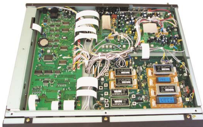
Figure 4—The roofing filter installed in a Mark V FT-1000MP.
