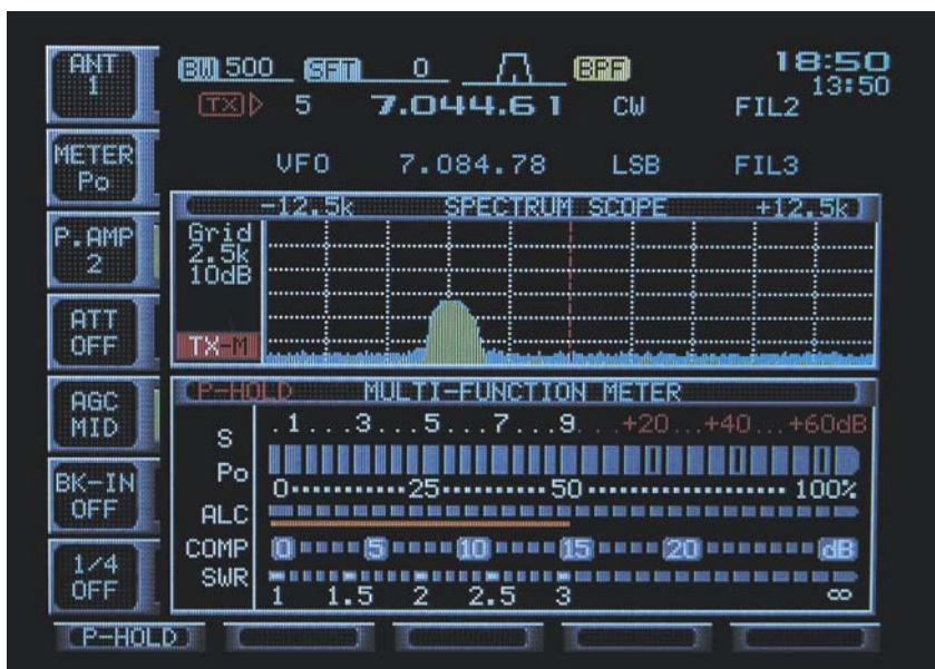
Figure 4—Close-up of the ICOM IC-756PROIII display in MSCOPE mode viewing the spectrum scope and the multifunction meters. Note the dual clocks.
