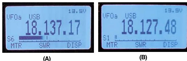
Figure 2—My transceiver display before applying the ICE 475-3 (A) and after (B). Notice that the S-meter display has dropped from S6 to S1.
