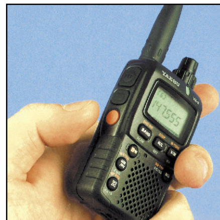
Figure 1—There’s the power button! The bright orange button on the side panel is hard to miss. The placement and increased resistance of the on/off key is a good feature, allowing added space on the front panel and minimizing accidental turnings on and off.
