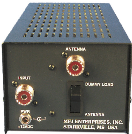
Figure 3 —The rear panel of the MFJ-267 wattmeter and dummy load. Notice that the switch sending the input to the antenna or the dummy load is here, making the user reach around.
